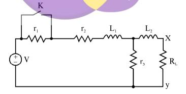
(f) In figure with switch open, steady state is reached with v=100sin314t volts. The switch is closed at t=0. The circuit is allowed to come to steady state again. Determine the steady state current and complete solution of transient current.
